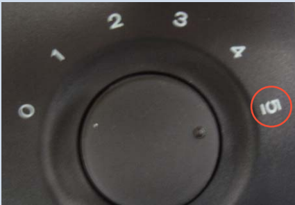
All humidifiers with an underlined 5 are compatible with J-tube chamber part number 1003758.
